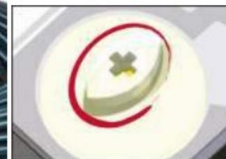
Raised inlets ensure that sediment deposits at the bottom of the tube do not enter the emitter.
